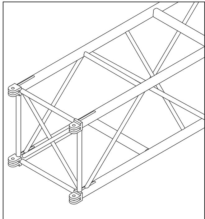
LOADING FIGURES show maximum loads between supports in addition to self weight of truss. Information extracted from structural report by The Broadhurst Partnership. \* Denotes load limited to suit maximum shear capacity. All loads include a 20% overload factor for dynamic effects.
